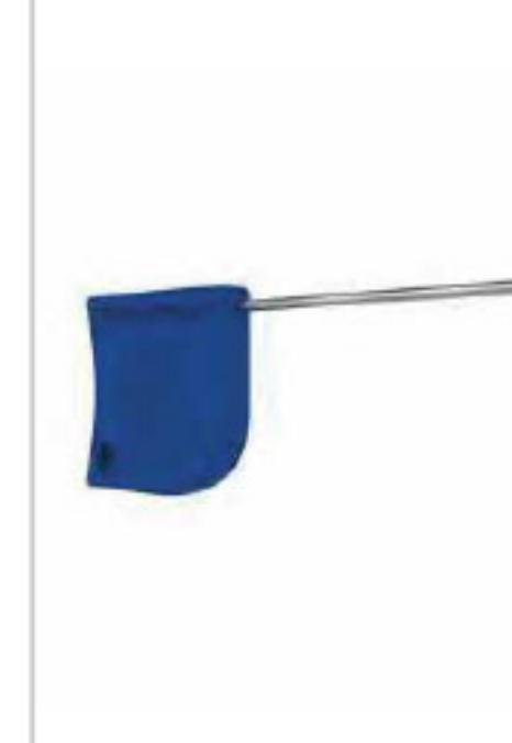
The Setting Key allows Gripple tensioners to be repositioned on the wire before tension is applied. To use, simply insert the key into the small hole adjacent to the main channel, releasing the roller and allowing the tensioner to move freely.
