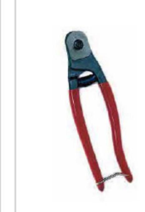
The Wire Cutters are suitable for cutting high tensile wire or wire rope up to 4 mm. The spring loaded non-slip handles make it easy to use and the hardened steel jaws deliver great results.
