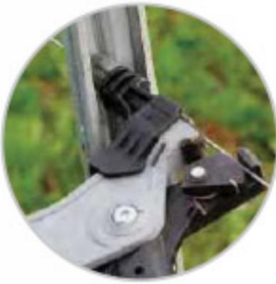
The Torq Tool is lightweight, compact and tensions up to 6 mm Gripple tensioners. Designed with an in-built gauge, the tool measures the tension you wish to apply. With the addition of the Adaptor, the Torq Tool can be used in recessed applications.
